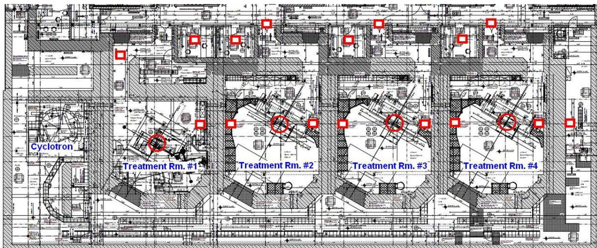
Figure A.1.1. Showing the treatment rooms of the WPE facility, which is based on an IBA Proteus 230 room temperature proton cyclotron, one fixed beam Treatment Room (#1) and three gantry Treatment Rooms (#2 - #4). The circles and rectangles indicate the radiation sources (proton impact points) used for radiation safety calculations and locations of neutron and gamma dose equivalent rate measurement respectively.
