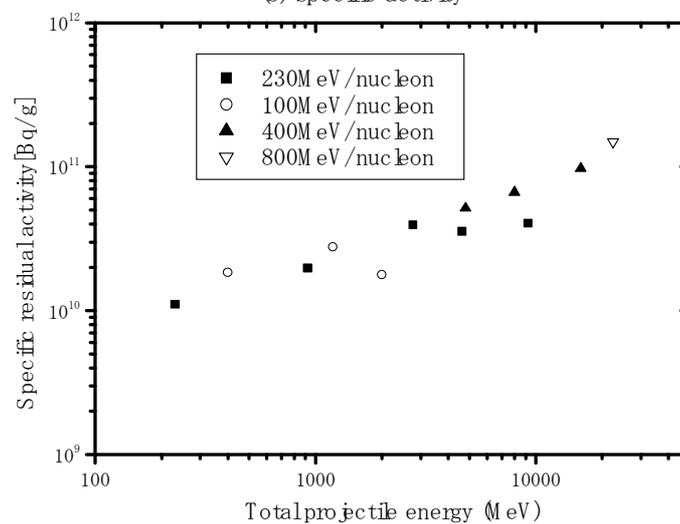
3630 Figure 5.9. Projectile energy dependence of total residual activity and specific residual activity induced
